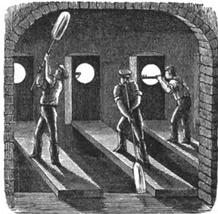
FIG. 18.—Blowing Cylinder Glass.
