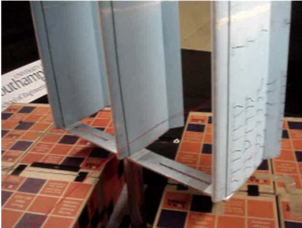
Figure F.11 – Container - Sail interaction study. the gap between the boxes and the base of the wing replicates the full scale gap of 2 metres. Note the red wire which was used instead of the smoke to visualize the flow near the gap; unfortunately this intrusive method had limited effectiveness.
