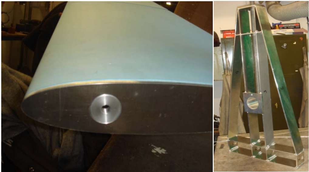
Figure F.2 – Model manufacture: wing with stock (left); and base (right)
