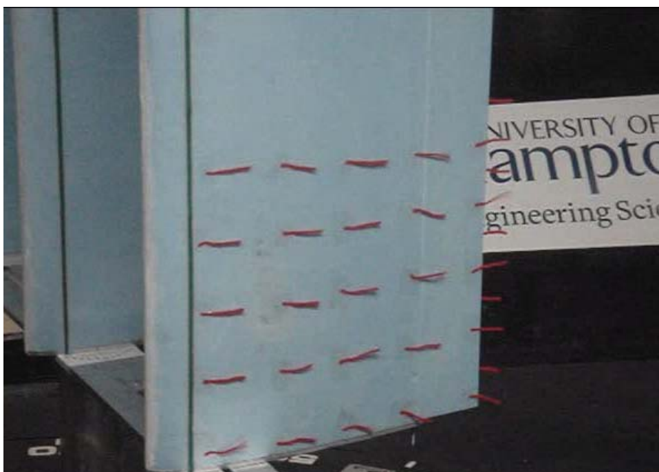
Figure F.10 – Low Reynolds number testing. V_a = 8 \text{ ms}^{-1} , \text{AoA} = 14 degrees. Here the tufts are aligned with the flow and are attached to the surface. Observing the bottom row is possible to note the end vortex coming off the wing; the first two tufts of this row are separating from the surface due to the interference of the bottom bar
