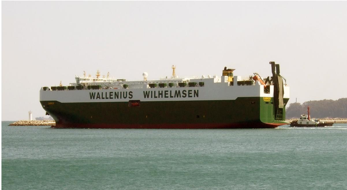
The LCTC (Large Car Truck Carrier) m/v CARMEN with her 227.8 meters and 74,258 gross tonnage has a capacity of 7,879 cars or a combination of 3,508 cars and 432 buses. The vessel is built to the highest class
