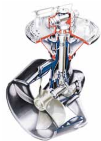
SCHOTTEL Rudder propeller (Z-drive)
