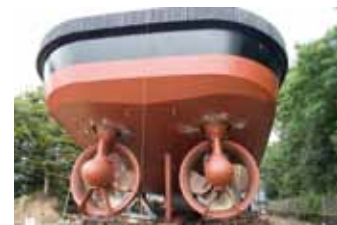
Twin-screw propulsion with ducted propellers
