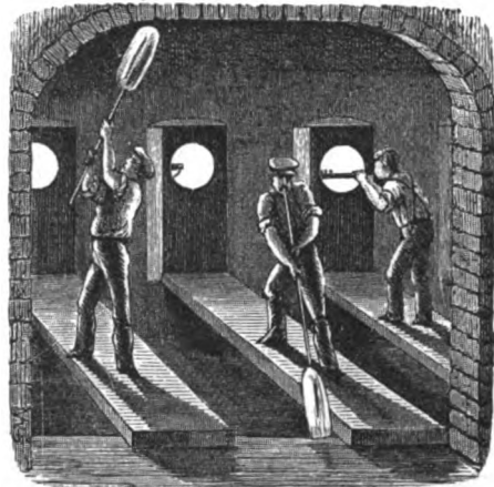
FIG. 18.—Blowing Cylinder Glass.
