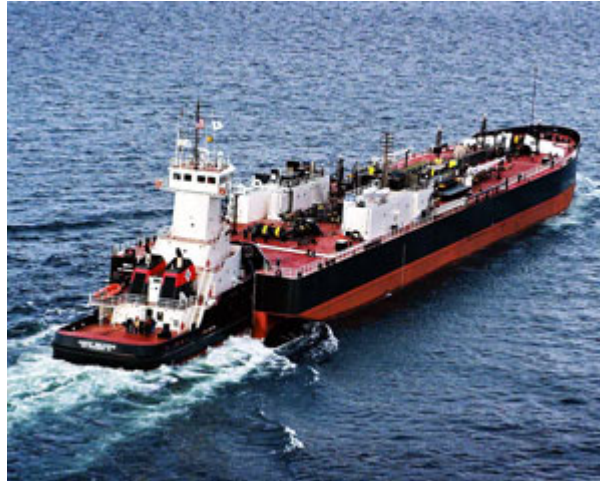
Figure 12. Articulated Tug/Barge Used by Crowley Maritime for Petroleum Movements.
