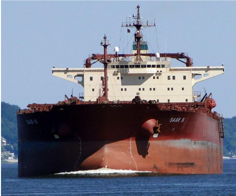
Bulk Carrier GT:63,153 tons Summer DWT:138,808 tons LOA:266m Beam:40m Draught: 15m
