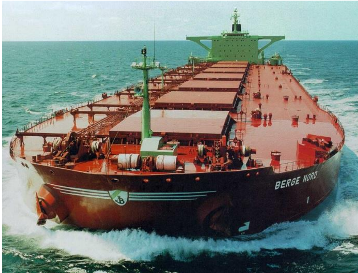
Ore Carrier GT:107,512 tons Summer DWT:218,283 tons Length:305m Beam: 54m Draught:11 m
